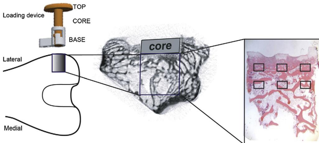
**Fig. 2.** Schematic of loading device (left) on femur and lateral view of distal femur showing device position and core location (middle) and location of the underlying cancellous bone (right) with histological areas of interests.
