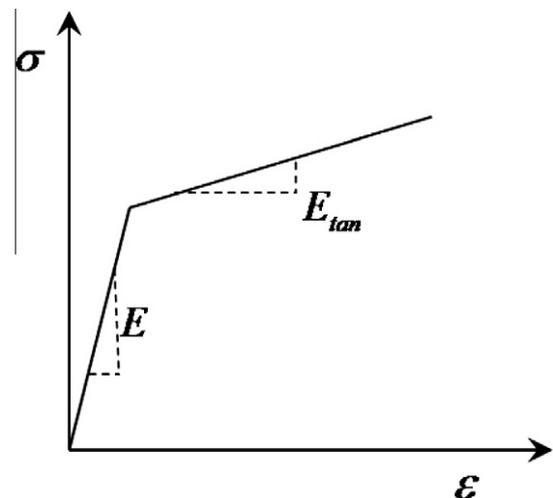
Fig. 1. Bi-linear stress–strain relation.
