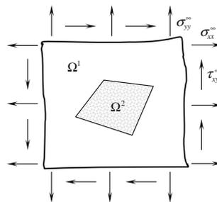
Fig. 1. An infinite plate containing a non-ellipsoidal inclusion.
