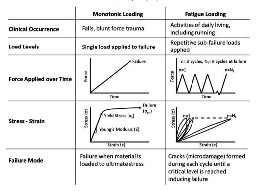
Fig. 1. Comparison of monotonic and fatigue loading. In monotonic loaded samples, force is increased until the sample fails. In fatigue, a repetitive sub-failure load is applied creating damage that eventually coalesces to cause failure.
