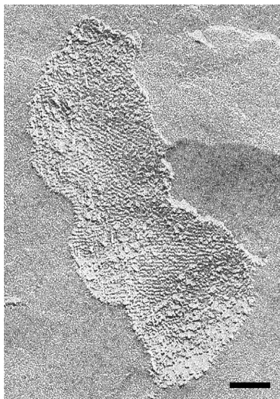
Fig. 1. A freeze-fracture image of a mosaic carboxylase 2D crystalline sheet grown below the phase transition temperature of the added phospholipids (DMPC). The freeze-fracture results demonstrate that the carboxylase crystals are indeed constituted of ordered protein. The scale bar is 100 nm.
