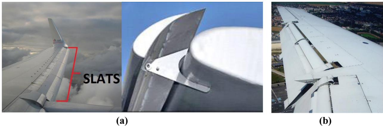
Fig. 1. Similar to an airplane landing mechanism, aerodynamic features are inspired to reduce wind loads on buildings: (a) slats; and (b) flaps.
