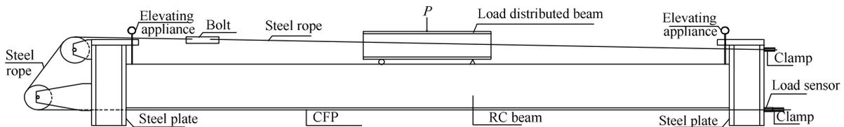
Fig. 2 Schematic diagram of pre-stress application
