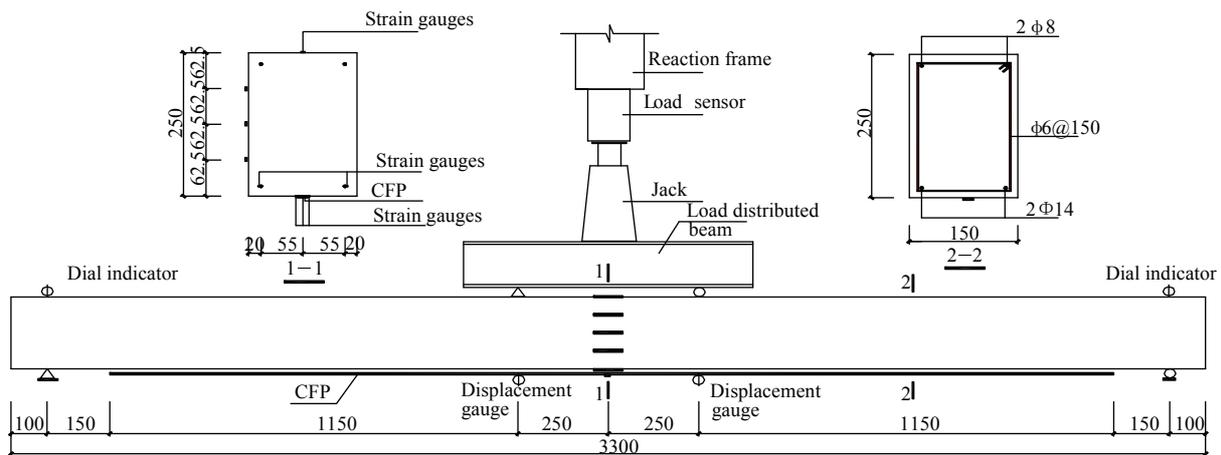
Fig. 1 Schematic diagram of loading device, strain gauge allocation and rebar arrangement (mm)
