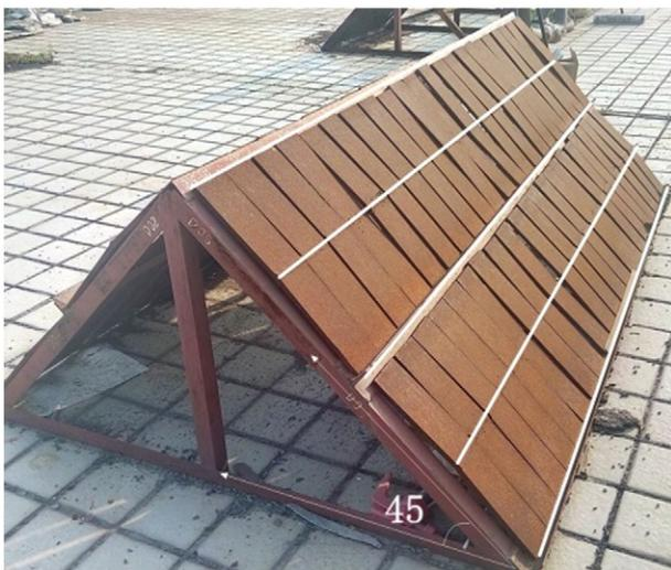
Fig. 1. Condition of accelerated corrosion experiment.
