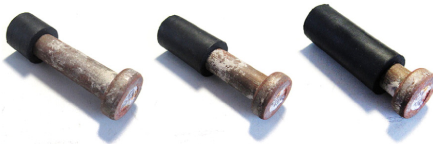
Fig. 1. Rubber-sleeved studs with different rubber sleeve heights.
