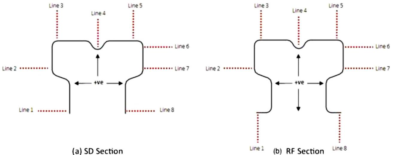
Fig. 2. Locations of laser lines for RF and SD sections.
