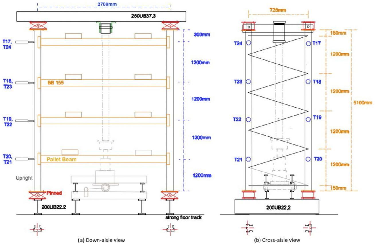
Fig. 1. Test Setup - Frame orientation, bracing dimensions and transducer locations.
