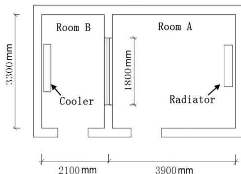
Fig. 1. Dimensions of climate chamber.
