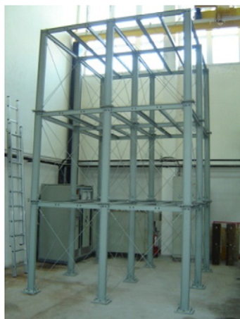
Fig. 2. The investigated steel building model and its dimensions.
