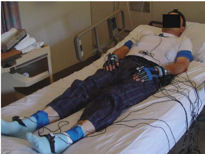
Fig. 2. The multisensor physical activity micro-measurement system on a participant.
