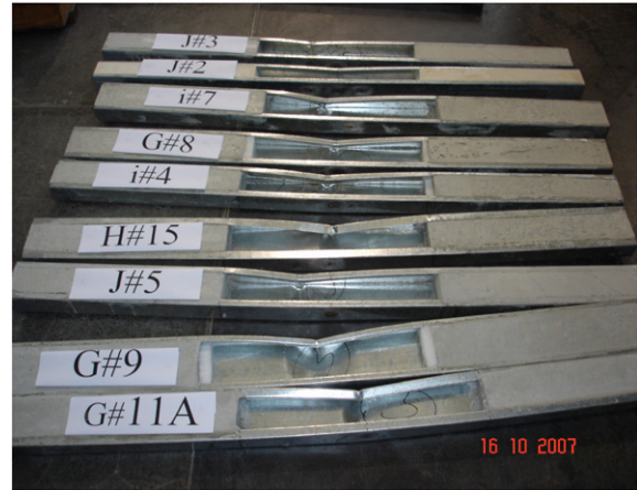
Fig. 1. Sample tested sections.
