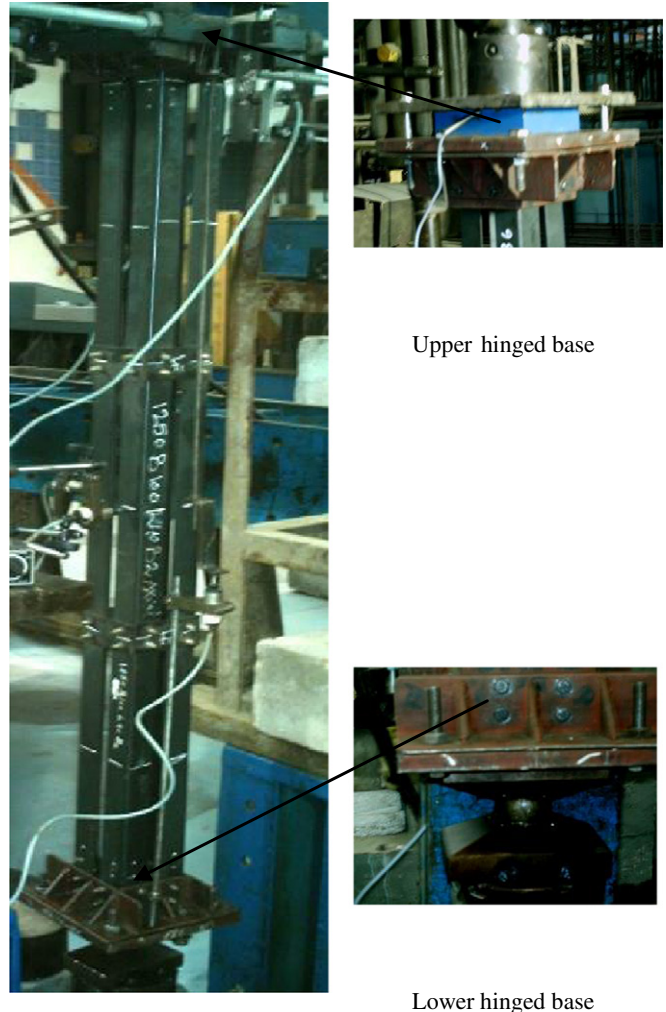
Fig. 1. Test setup. a) Upper hinged support. b) 4 Steel bars. c) Upper end restrains ( U_x, y & R_z ). d) Lower hinged support.
