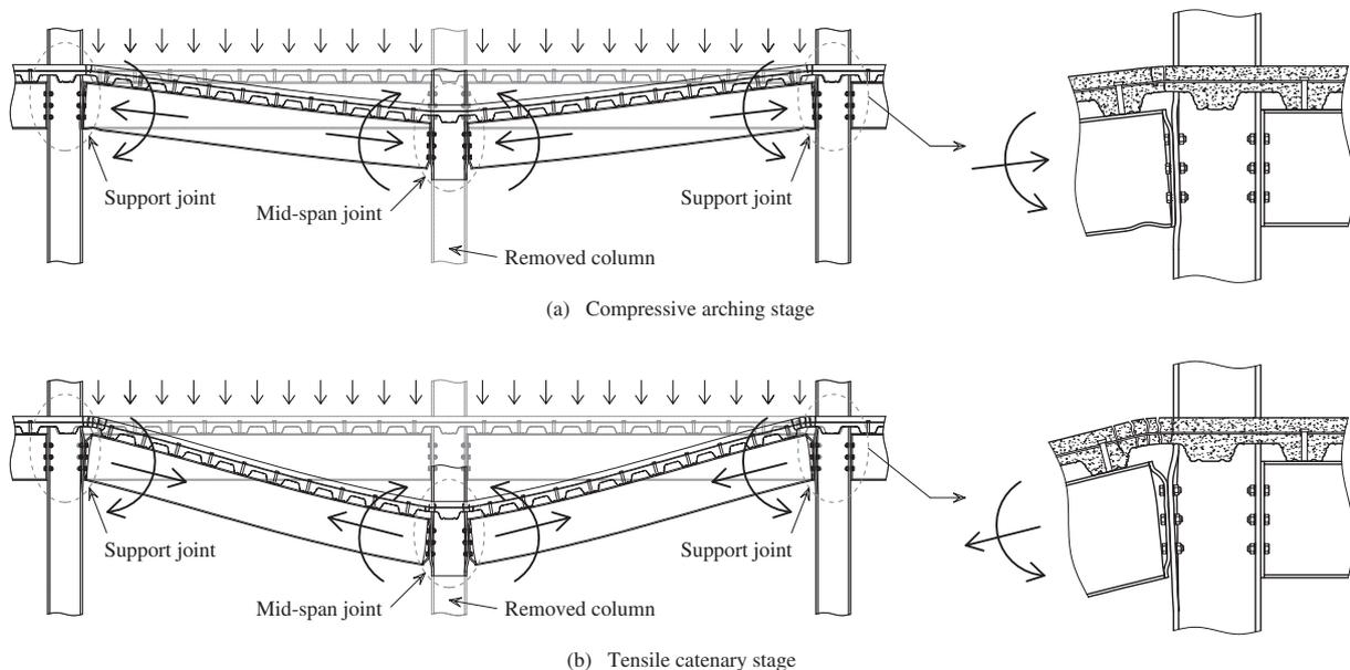
Fig. 1. Double-span beam condition created by column removal.
