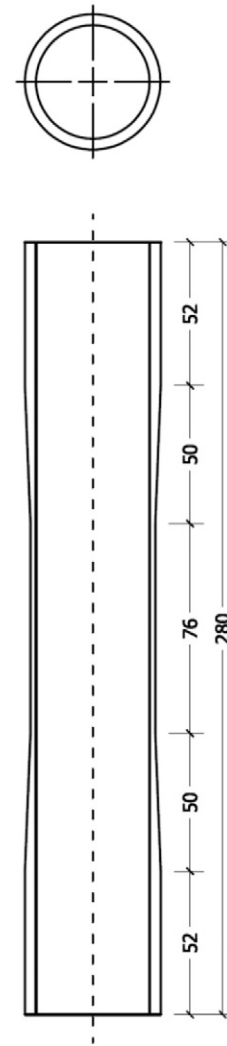
Fig. 1. Geometry of the tested tubular specimens (all dimensions in mm).
