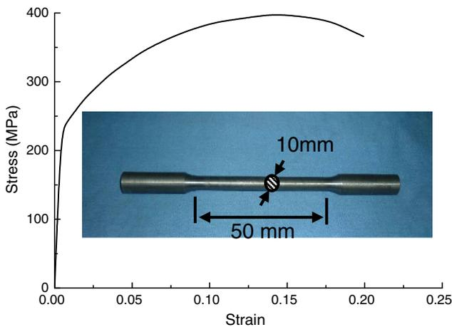
Fig. 2. Stress-strain curve of Q235 steel.
