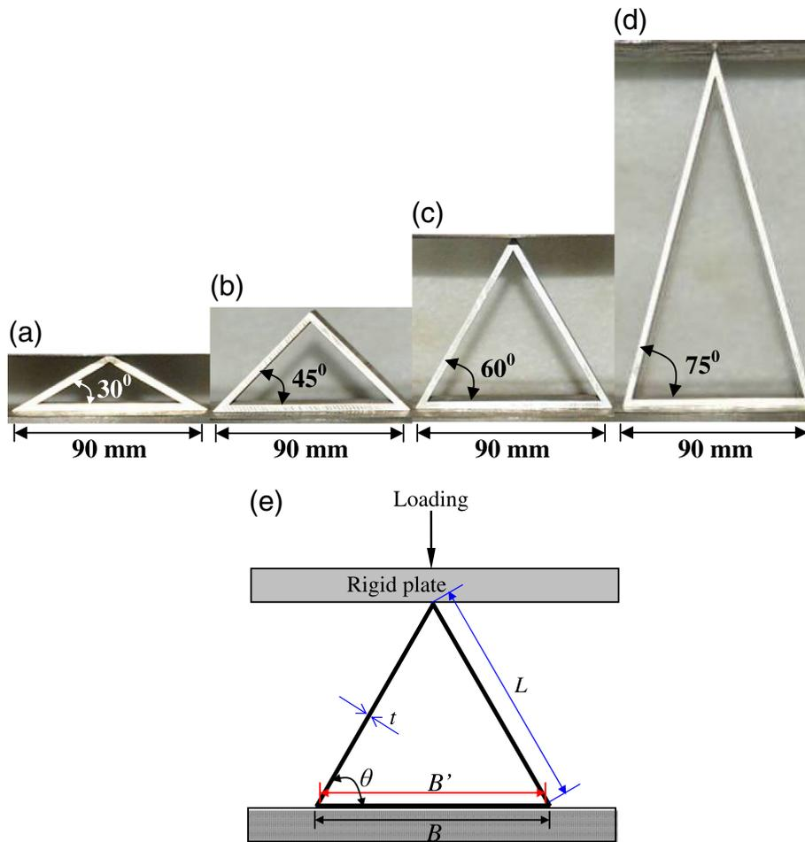
Fig. 1. Isosceles triangular tubes with base angles of (a) 30°, (b) 45°, (c) 60° and (d) 75° and (e) the sketch map of lateral compression.
