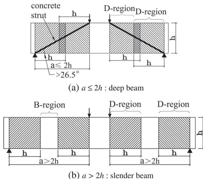
Fig. 1. Comparison between deep beams and slender beams in ACI 318-05.
