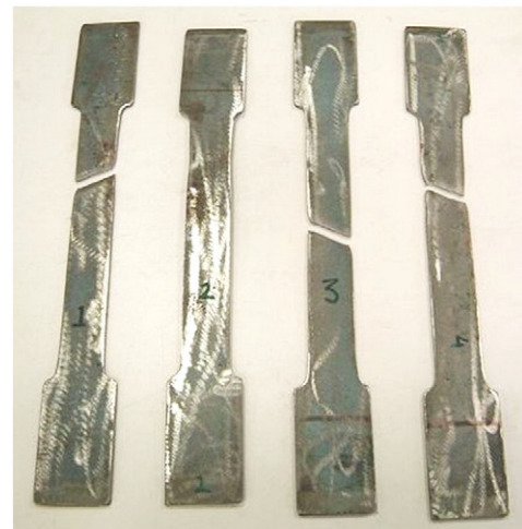
Fig. 2. Typical failure mode for tensile coupon.
