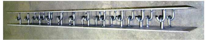
a) SCS sandwich beam with J-hook shear connectors (before casting)
