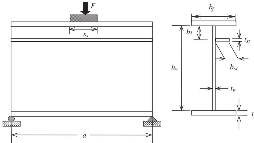
Fig. 1. A longitudinally stiffened plate girder under patch loading.
