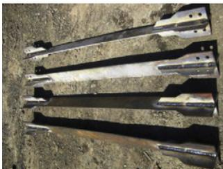
(b) The surfaces of inner cores were wrapped with plastic film
