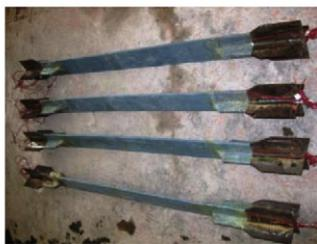
(c) The inner cores were located in steel tubes
