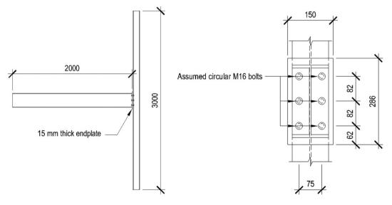
Fig. 3. The endplate connection dimensions.
