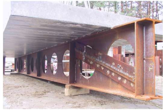
Fig. 4. Specimen of cellular composite beam with wide openings (RFCS project) [6].
