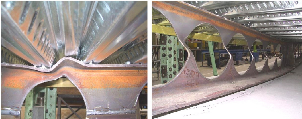
Fig. 3. Failure modes of composite cellular beams: Vierendeel bending (left), web-post buckling (right).
