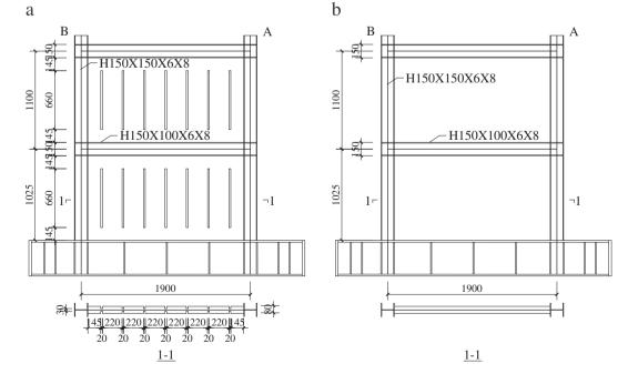
Fig. 1. Dimensions of specimen: (a) specimen no. 1; (b) specimen no. 2 (dimension in mm).
