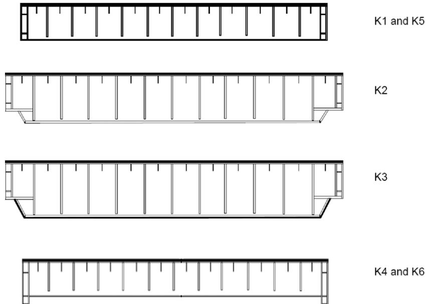
Fig. 2. Types of crane runway girders.
