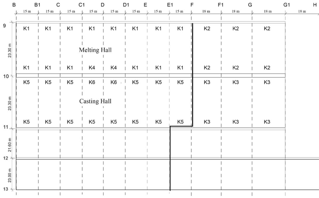
Fig. 1. Plan view of the crane girders.
