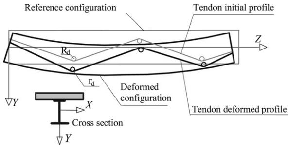
Fig. 1. Beam model with external prestressing.
