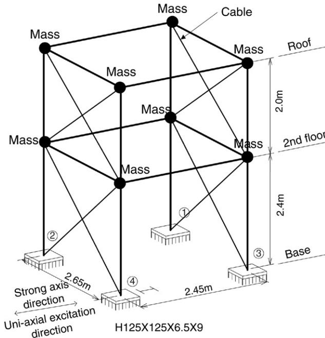
Fig. 1. Dimension and loading conditions of test frame.
