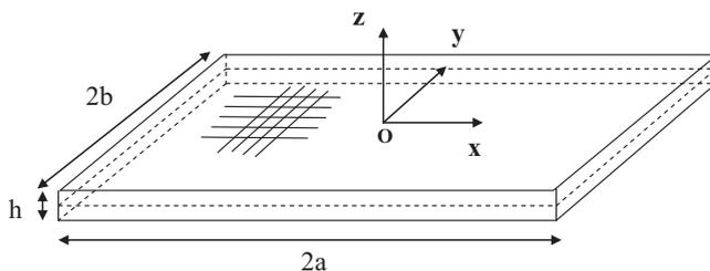
Fig. 1. Orthotropic plate.
