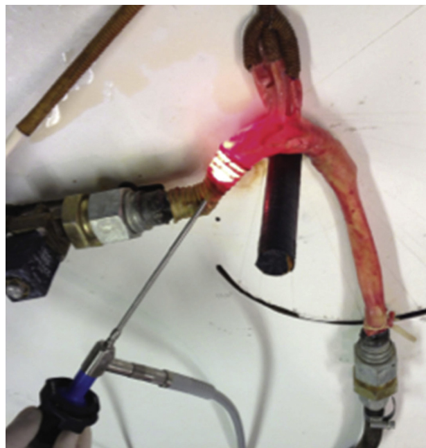
Fig 1. Benchtop closed-system pulsatile flow model. A graft is anastomosed to the distal segments of the aortic arch side branches. To monitor the procedure, a 5-mm angioscope connected to a camera was introduced into the ascending aorta.
