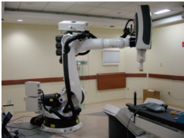
FIGURE 1. Cyberknife device with a linear accelerator mounted on a robotic arm.
