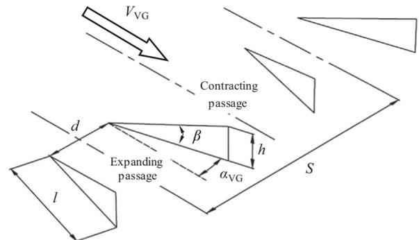
Fig. 2. Sketch of VGs:  $V_{VG}$  is the local velocity;  $d$  is the leading edge spacing in a pair of VGs;  $l$  is the length of VGs;  $\alpha_{VG}$  is the angle of attack of VGs with respect to the local velocity;  $h$  is the height of VGs;  $S$  is the spacing of adjacent pairs of VGs;  $\beta$  is the leading edge angle of a VG equaling to  $\alpha_{VG}$  in this study.
