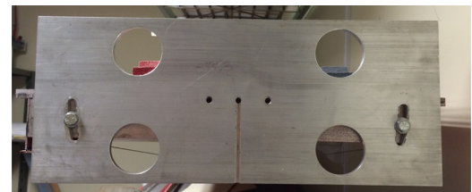
Fig. 2. End plates with long slots for adjustment in wind coordinates.
