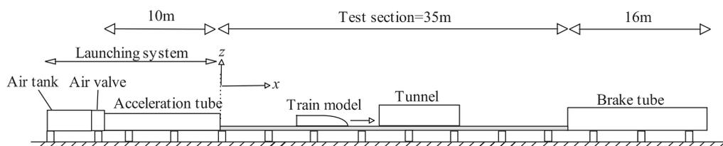
Fig. 1. Schematic figure of the experimental facility.
