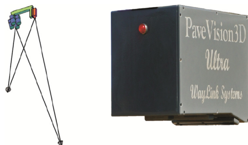
Fig. 2 – Laser imaging principle (WayLink).
