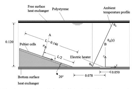
Fig. 2. Schematic representation (not in scale) of a portion of the investigated area (all the measurements are in metres).
