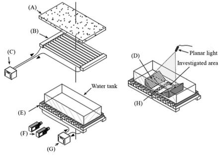
Fig. 1. Experimental apparatus: (A) polystyrene sheet, (B) free surface heat exchanger, (C) free surface thermostat, (D) valley model, (E) bottom surface heat exchanger, (F) cameras, (G) bottom surface thermostat and (H) rectangular-shaped electric heater.
