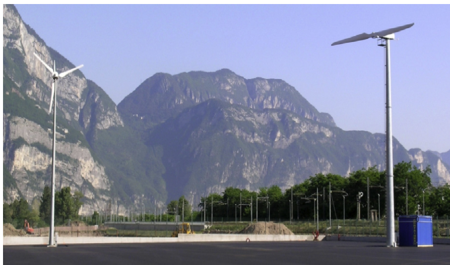
Fig. 1. GW turbine, 12 kW, fixed-speed, two bladed, downwind (right); JT turbine, 20 kW, three bladed, upwind (left); the view is from South to North.
