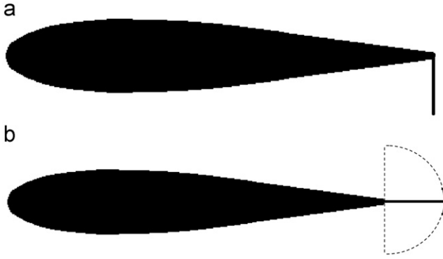
Fig. 1. Static gurney flap (a) and dynamically deployed trailing-edge flap (b).
