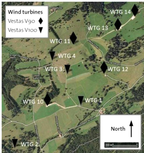
Fig. 1. Layout of the central portion of the wind farm located in complex terrain in western Switzerland.
