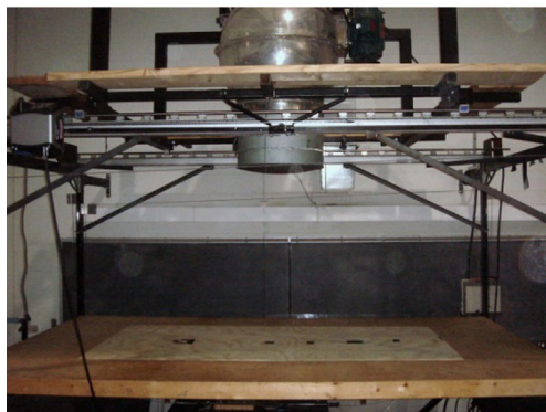
Fig. 1 . Microburst simulator at Iowa State University: photo and schematic.
