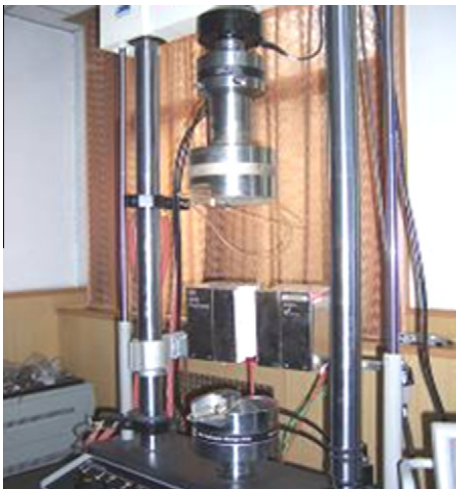
Fig. 1. MTS810 servo-controlled rock mechanics testing machine and MTS652.02 high temperature furnace.
