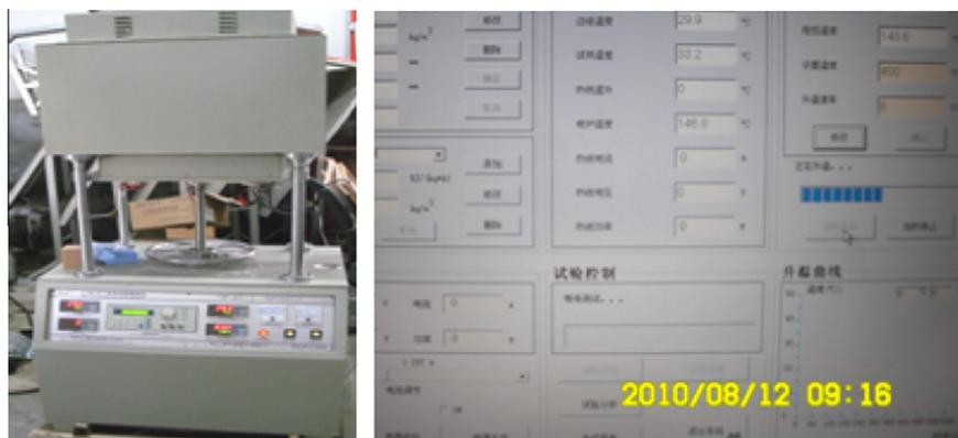
Fig. 1. DRX-II coefficient of thermal conductivity measurement equipment and the test control system.
