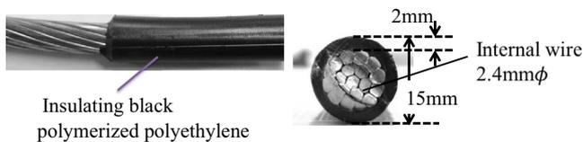
Fig. 1. The photographs of typical covered copper cable sample.
