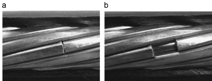
Fig. 2. The photographs of artificially made disconnected copper wire portion with the snapped space of (a) almost 0 mm, (b) 3 mm. THz imaging was carried out after the opaque polyethylene insulator was attached again.
