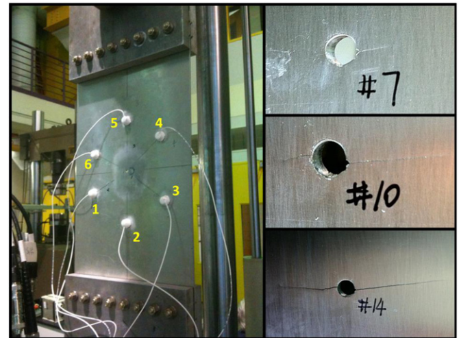
Fig. 1. Aluminum plate with attached transducers (numbered 1–6) mounted in the testing machine prior to fatiguing (left), and photographs of fatigue cracks corresponding to data sets 7, 10 and 14 (right). The front of the plate is the transducer side; crack photos are from the back of the plate.
