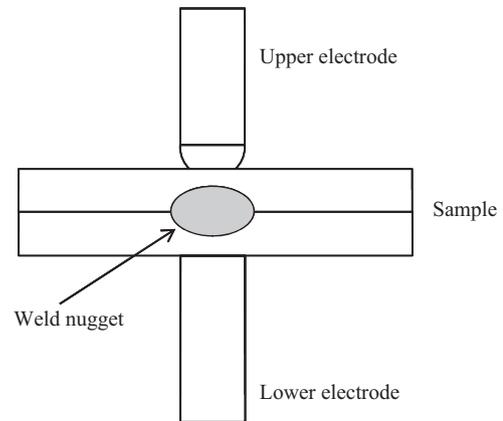
Fig. 3. Schematic diagram of the electrodes of the welding machine.
