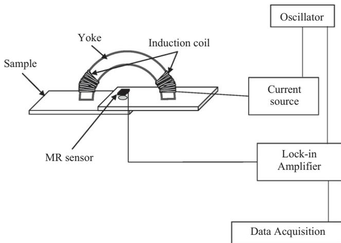
Fig. 1. Schematic diagram of the developed magnetic flux leakage testing system.
