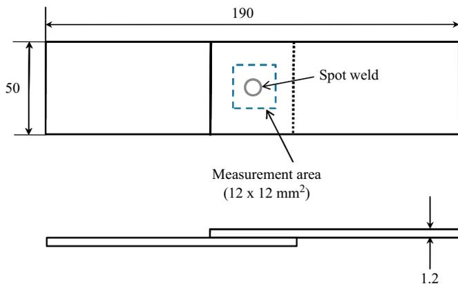
Fig. 2. Shape and dimensions of the welding spot specimen. Measurement area is 12 mm × 12 mm.
