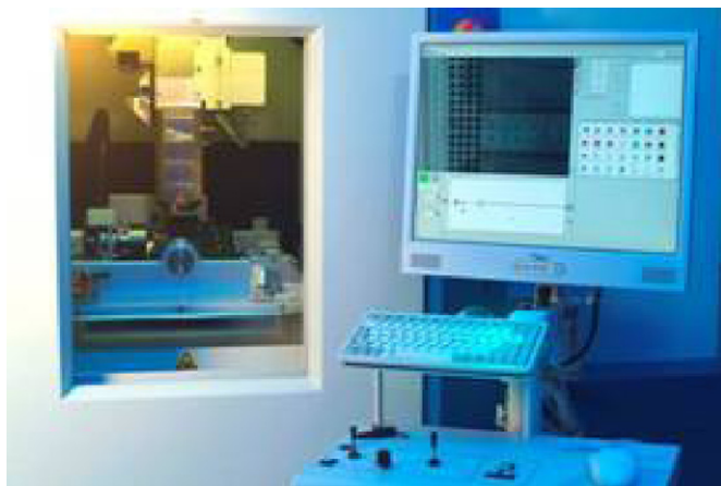
Fig. 2. A Nanofocus Focus FOX 160.25 X-ray imaging system.
