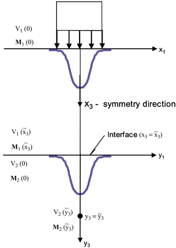
**Fig. 1.** Propagation of a Gaussian beam in a symmetry direction of anisotropic solid. Two anisotropic solids have a normal interface with respect to the beam path.
