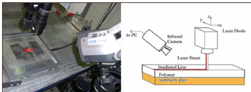
Fig. 1. Equipment for IR image recording during laser welding.
