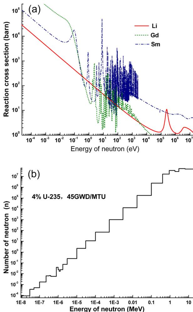
Fig. 1. (a) Neutron cross section of three kinds of neutron absorbers ( $\text{LiF}$ ,  $\text{Sm}_2\text{O}_3$ , and  $\text{Gd}_2\text{O}_3$ ). (b) Neutron spectrum of spent fuel (4 wt%  $^{235}\text{U}$ , 45 GWD/MTU, cooling time 5 years).
