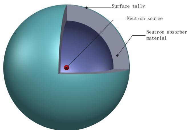
Fig. 2. The spherical shell model used for calculation.
